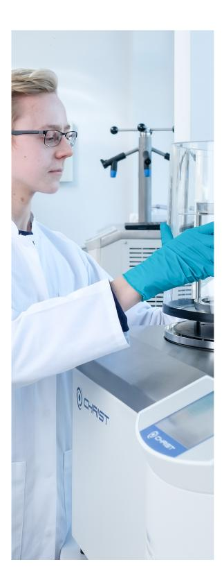
Freeze drying is not only used for water-based materials. Typical examples include HPLC fractions with organic or inorganic solvents, such as acetonitrile, TFA and other alcohols, or other products with t-butanol, DMSO, etc. The Alpha 3-4 LSCbasic is available in two defined packages, fully aligned to the requirements of freeze drying with solvents.
